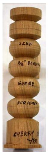
The beads to the left can be "rolled" with almost anything. A skew gives the best surface, but not much better than a sharp gouge. The shape iust above the skew-rolled bead is a cylinder flanked by groves made by my skew. This creates room for the bead rolling.
