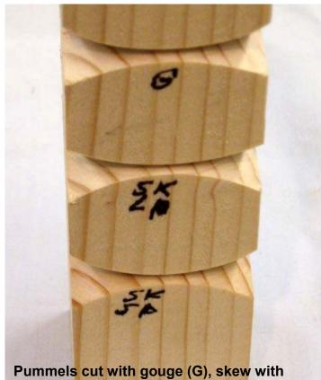
Pummels cut with gouge (G), skew with long point down, (SK LP), and skew with short point (heel) down (SK SP).
