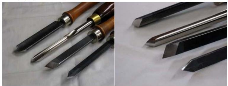
Basic set of spindle turning tools: 1 inch spindle gouge, 1/2 inch spindle gouge, 1/2 inch skew, and parting tool. The picture on the right shows the tools rotated 90 degrees to show the grind profile which can vary quite a bit, and is less important than the sharpness of the tool. These are all cutting tools, although the skew can be used on its side as a negative rake scraper if you don't mind sharpening it often.
